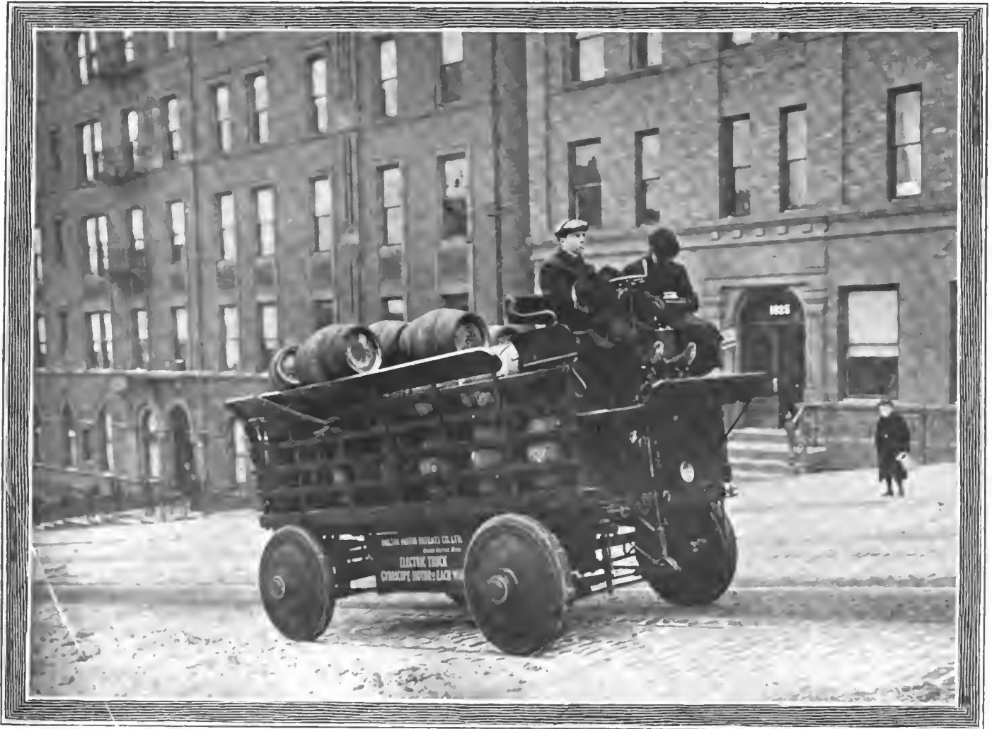
FOUR-WHEEL-DRIVE TRUCK CLIMBING NEW YORK'S STEEPEST HILL WITH FOUR-TON LOAD IN A HEAVY SNOWSTORM.
